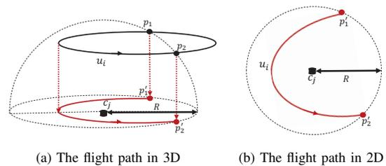
Fig. 3: Mapping flight paths from 3D to 2D plane
